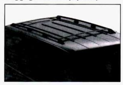
If you have the luggage carrier, you can load things on top of your vehicle. The luggage carrier has slats attached to the roof, side rails, and tiedowns.
